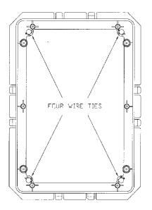
HD loudspeakers. Do not fill the holes of the grille with paint. The grille is constructed of aluminum with a perfectly even powder coat overall. This powder coat is an ideal primer.
